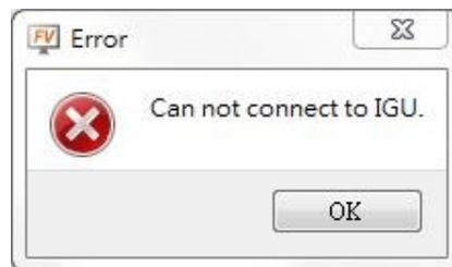
Figure 9 Error message for IGU-FvRT (USB Dongle) was not detected
