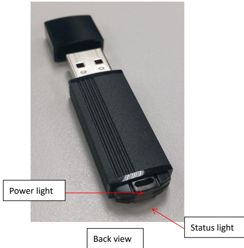
Figure 8 The appearance of IGU-FvRT (USB Dongle)
