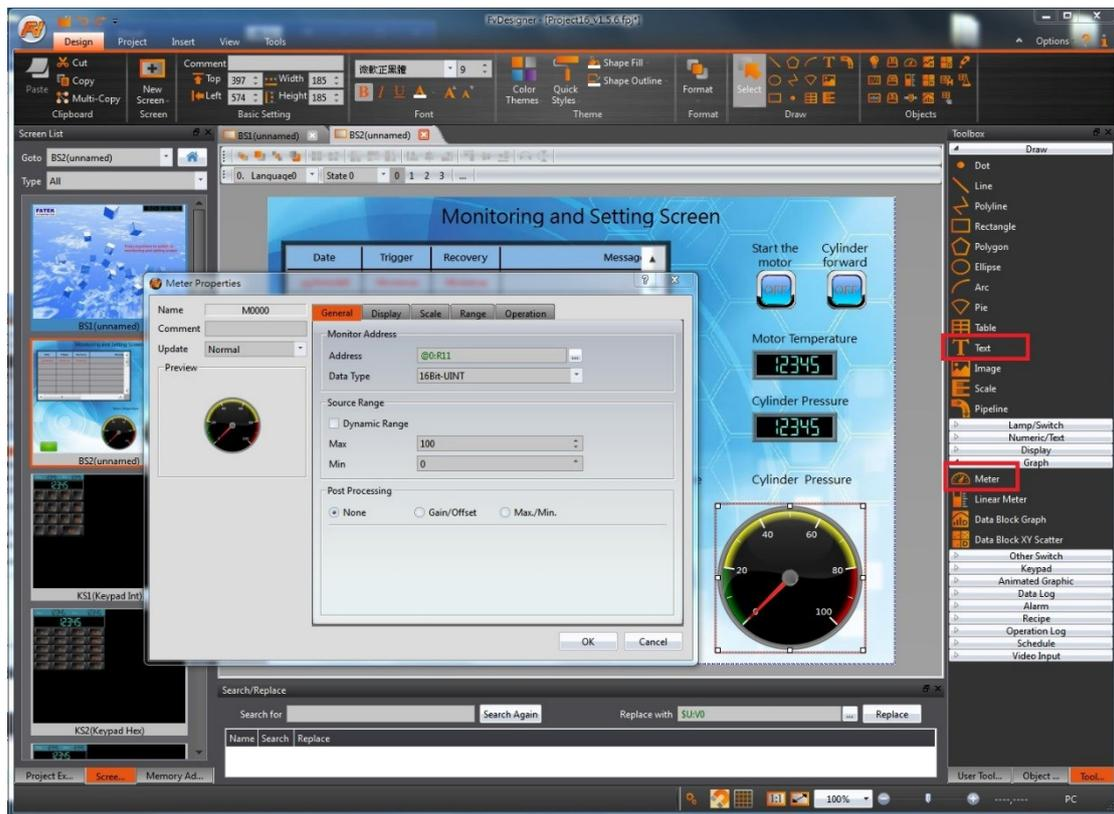
Figure 39 Add text and meter objects
