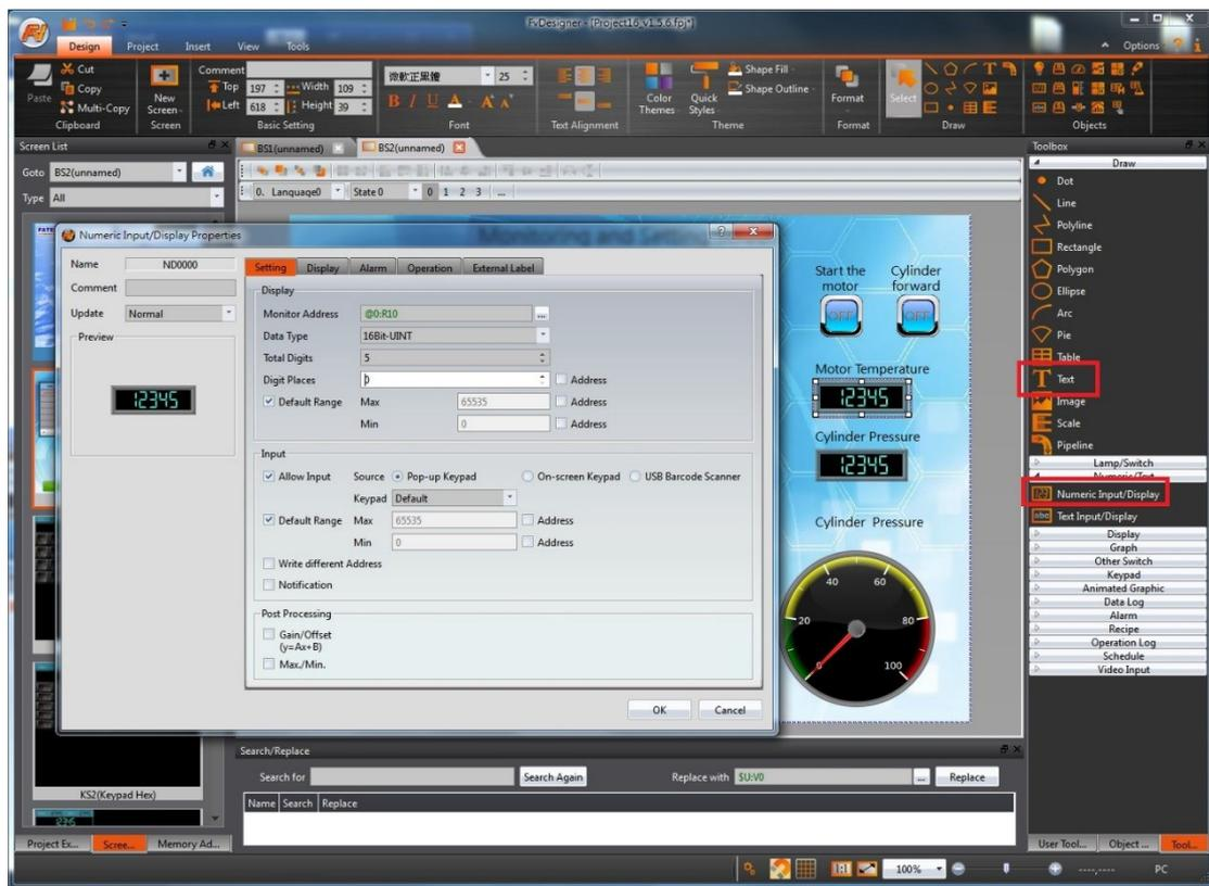
Figure 38 Add text and numeric/input display objects
